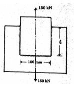
Two plates are joined together by means of single transverse and double parallel fillet welds as shown in figure given above. If the size of fillet is 5 mm and allowable shear load per mm is 300 N, what is the approximate length of each parallel fillet?
