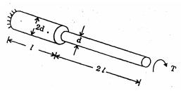
What is the total angle of twist of the stepped shaft subject to torque T shown In figure given above?
